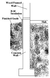
R-10 Slab insulation 2 ft in depth
