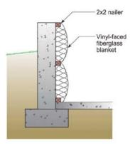
Continuous Interior R-10 Blanket Insulation in Basement
